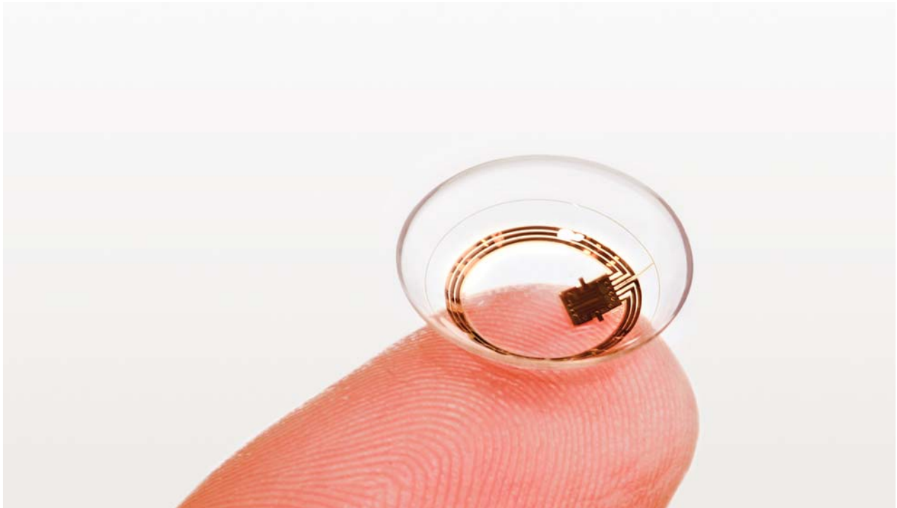
1, 2. Sensimed's Triggerfish lens features highly sensitive platinum strain gauges that record changes in corneal curvature that correspond directly with intraocular pressure.
