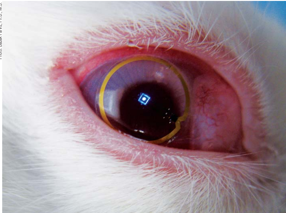
4. Placed on the eye of a live rabbit, this contact lens display is powered by a dipole antenna, showing bright emission from the on-lens pixel.
